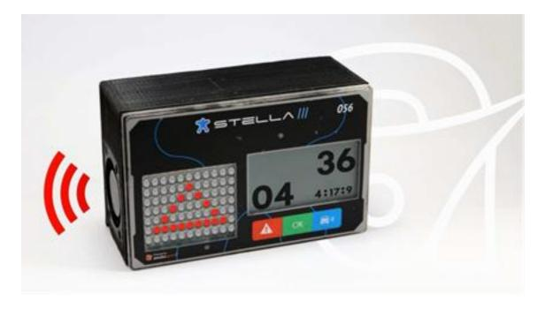
These alerts will inform the competitors that they are approaching a vehicle with some mechanical failure or rollover inside or outside of the track, to take all the necessary precautions while driving to prevent any accident.
