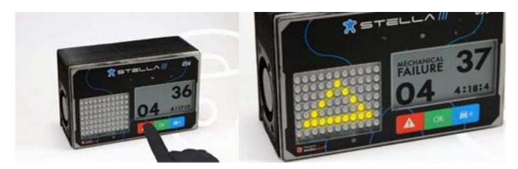
Competitors approaching your vehicle with mechanical failure will receive an alert on their led monitor, a symbol in the shape of flashing red triangle and an alert sound or a beep when they are within 300m of the damaged vehicle.
